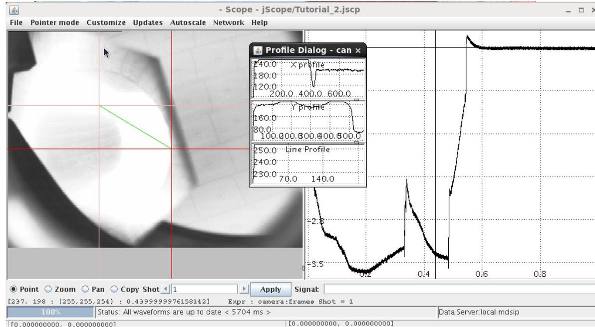
*jScope: tool for data access and display*
