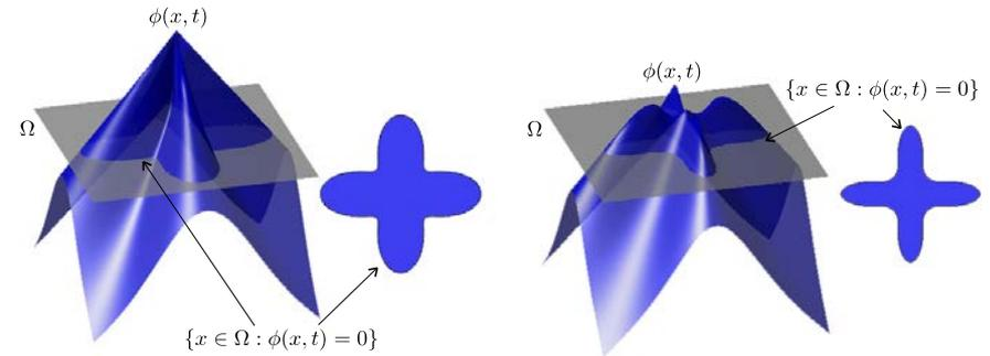
*In level set methods, the front is represented as the zero level set of a higher-dimensional function*
