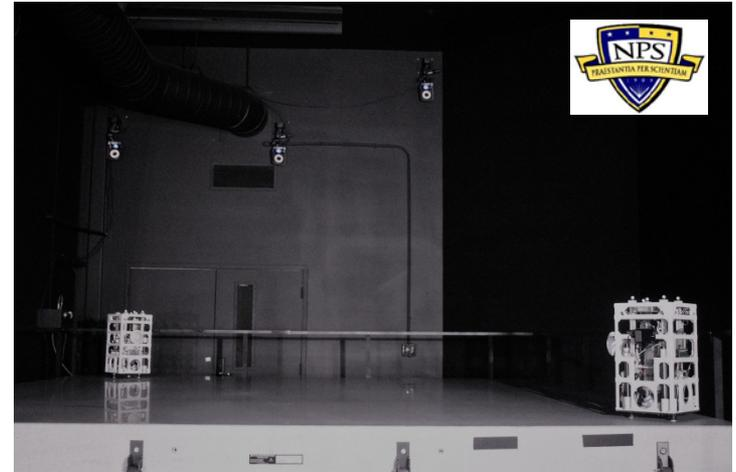
**NPS-POSEIDYN testbed, with Vicon motion capture, FSSs, and granite monolith at the Spacecraft Robotics Lab., NPS**
