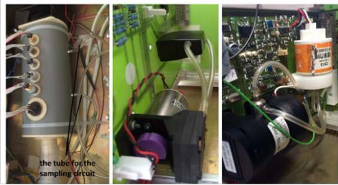
The sampling pump and the oxygen and carbon dioxide sensors
