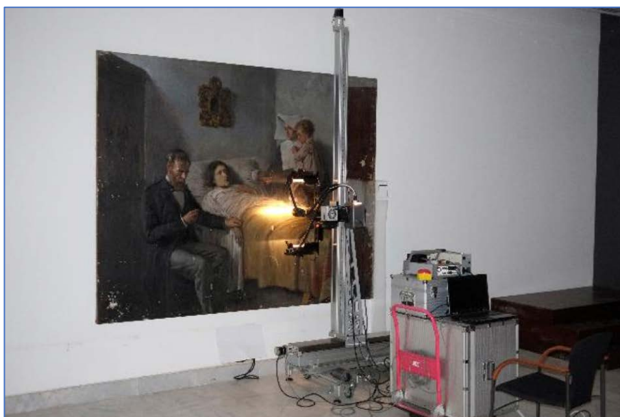
Fig. 1 - Example of hyperspectral image scanning at the Picasso Museum (Barcelona, Spain).
