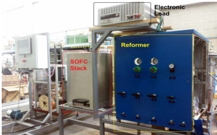
View of the Reformer connected with SOFC (SOFCOM EU Project)
