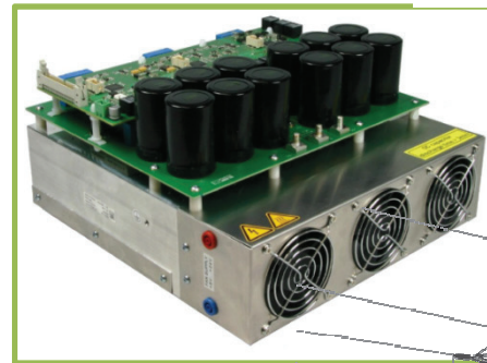
3-level neutral point clamped (NPC) Voltage Source Inverter (20 kW)
