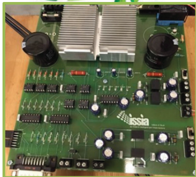
Half-bridge interleaved bidirectional converter for storage systems integration in building electrical power plants.
