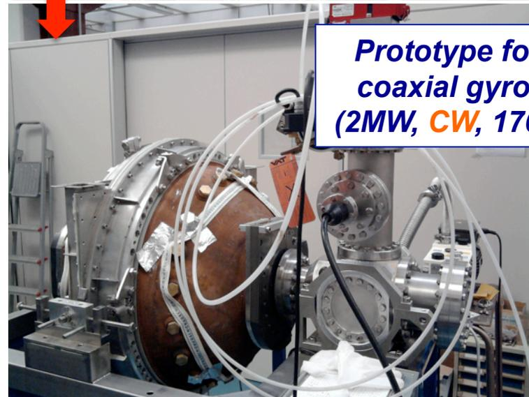
**Prototype for EU coaxial gyrotron (2MW, *CW*, 170GHz)**
