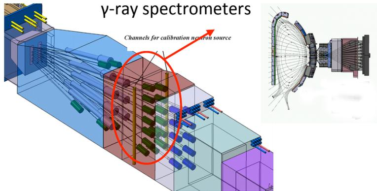
ITER Radial Neutron Camera with gamma ray spectrometers
