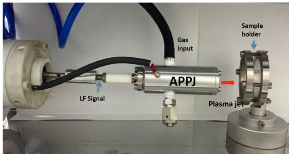
Bacteria inactivation by Atmospheric Pressure Plasma Jet (APPJ) treatment
