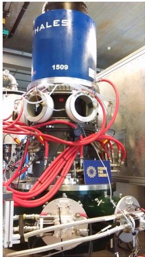
Testing prototype components and concepts for ITER (gyrotron and dummy load for high power operations)
