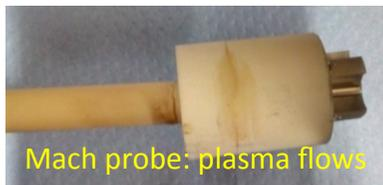
Measurements of electron density, temperature, plasma flows & potential. **Applications:** Physics studies
