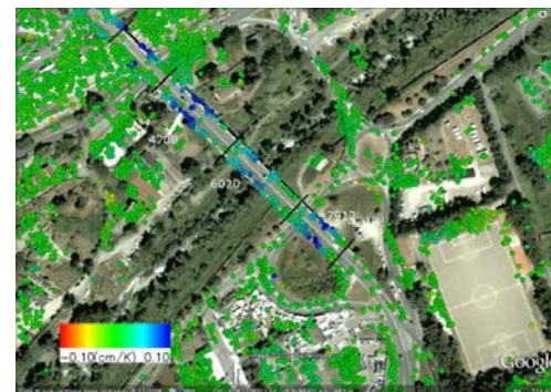
SAR monitoring of the displacement of a bridge
