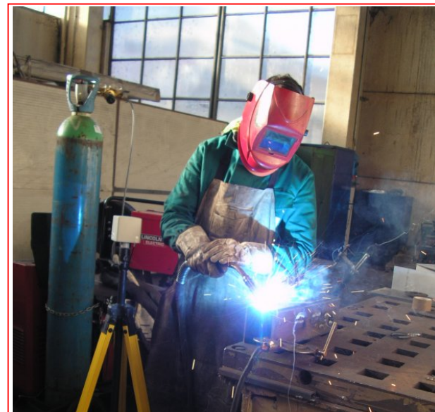
Measurement of electric and magnetic fields close to an industrial arc welding station
