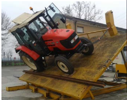
“Ergonomic approach for designing foldable ROPS”, OECD, 2017
