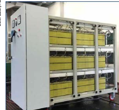
Example of Stationary Battery Pack under test
