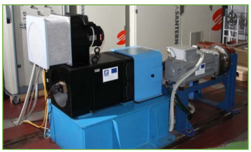
4-quadrant Dynamic Brakes for tests on driving cycles
